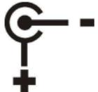
This will determine if you need to use the polarity reversal cable or one of the standard cables. This will allow you to use a pedal that has a positive center pin. Before you connect the cable from the unit, make sure you set the dipswitch to the appropriate voltage (9v or 12v).
