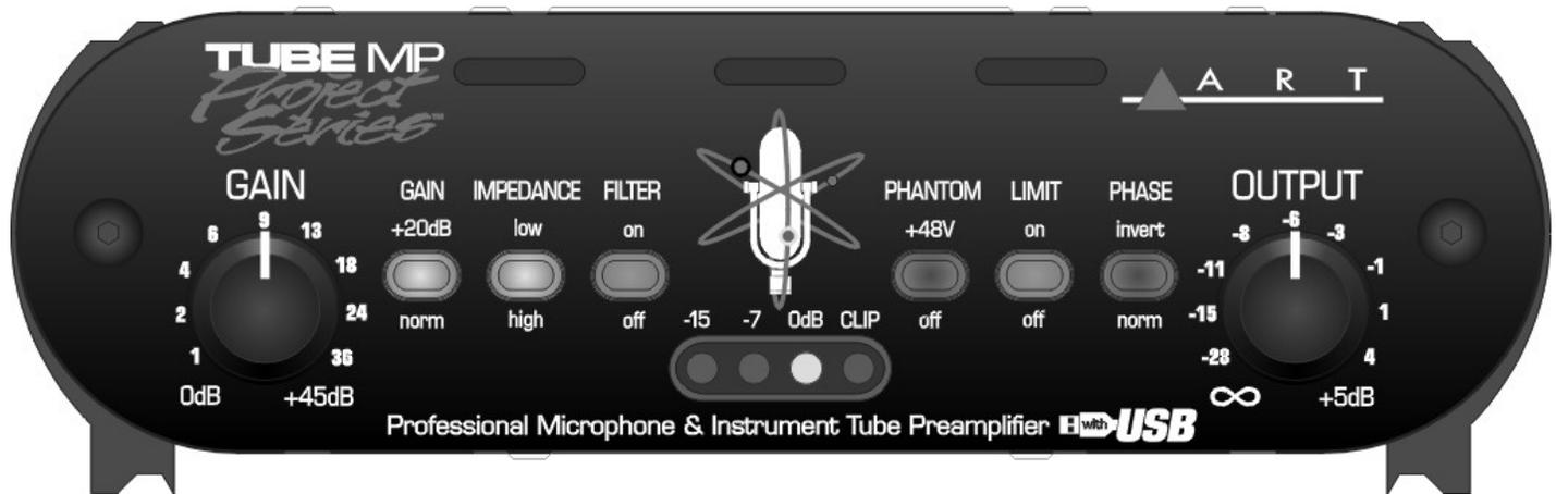
The **Gain** Control directly adjusts the input amplifiers giving you control over the dynamic range of your source. You get a 45dB gain range when using the XLR input and a 25dB gain range when using the 1/4" input. Set the control counterclockwise to minimum gain when connecting the inputs.
