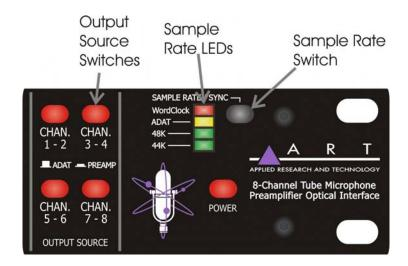
FIGURE 2 - Output and Sample Rate Section
