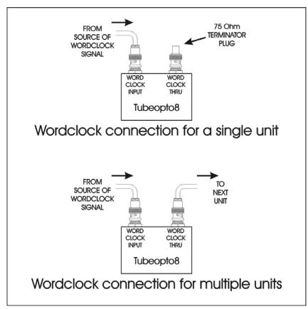
FIGURE 5 - Wordclock Connections
