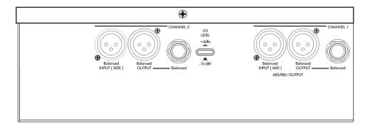
Figure 3 – Rear connections
