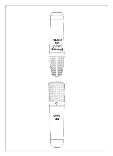
Figure 4 – Mid/Side Mic alignment
