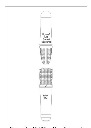
Figure 4 – Mid/Side Mic alignment
