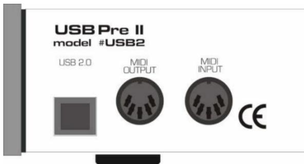
Use the **MIDI INPUT** and **MIDI OUTPUT** jacks to pass MIDI data back and forth between your computer and devices such as MIDI keyboard controllers, drum machines and sequencers. *The MIDI IN and MIDI OUT will show up as USB PRE II under your MIDI I/O selections.*
